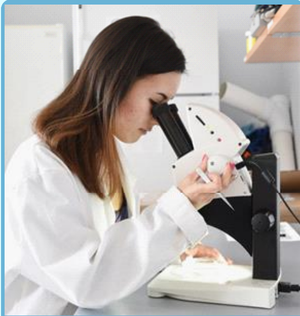
Photograph 3 SUNY Fredonia student technician looks for microbeads in a processed sample under a dissection microscope.
